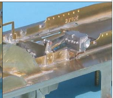
Lubricator drive, note 1.4mm copper rod and cut down base of cast lubricator
